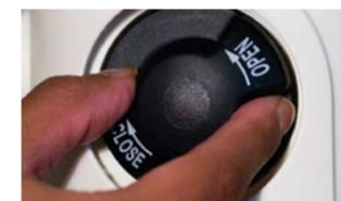
**4.1** To turn on the cylinder, slowly rotate the cylinder valve hand wheel anticlockwise at least one complete turn.
