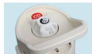
**2.7** Ensure the flow selector on top of the cylinder is set to zero and the cylinder valve hand wheel is turned off before connecting any equipment.
