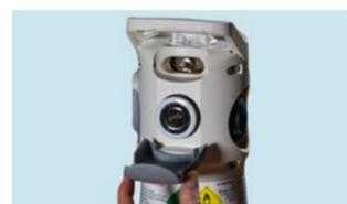
**2.8** Lower the hinged grey outlet cover to enable equipment connection.
