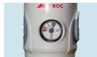
**2.3** Check the gauge to confirm the cylinder contents.
