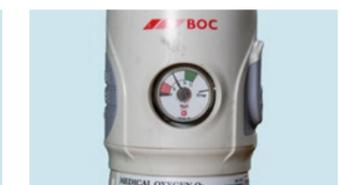
**6.8** Check the remaining cylinder contents using the gauge. If there is sufficient gas for further treatment, return cylinder to designated in use store. If the needle is in the red section return to the empty storage area.
