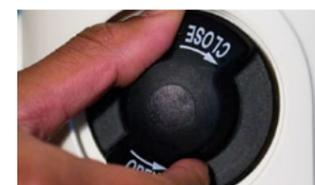
**6.2** Turn off the cylinder by rotating the cylinder valve hand wheel clockwise until it comes to a stop.
