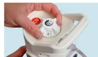
**3.3** Once the cylinder valve hand wheel is open, rotate the flow selector clockwise to the prescribed flow.
