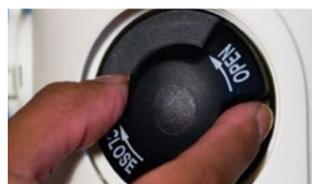
**3.2** To turn on the cylinder slowly rotate the cylinder valve hand wheel anticlockwise at least one complete turn.
