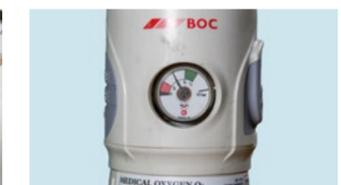
**5.4** Check the contents gauge at regular intervals, to ensure there is sufficient gas.
